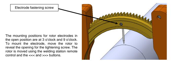
**CAUTION**: This screw is an M3 headless screw that must be tightened with care. It should not be manipulated with a ball driver hex wrench, which could damage the screw head! The Allen wrench required is provided.
