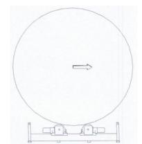
Figure 6 Wheel Brackets Too Close Together
