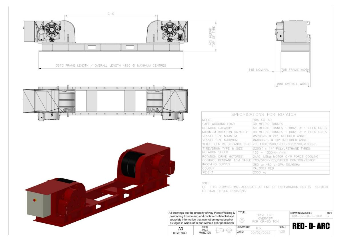
Figure 11 Drive Section GA Drawing & Specification
