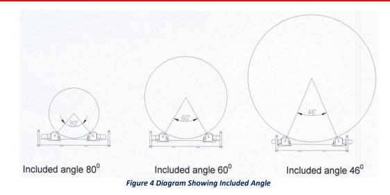
You can quickly calculate the distance that the wheel brackets need to be apart in order to achieve a  $60^{\circ}$  included angle. It is;
