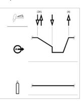
Welding current, like in step 4, to continue welding. When the main part of the weld is complete go to step 3. As shown here, again after the TIG torch trigger is quickly pressed and released from step 3A, it is possible to quickly press and release the TIG torch trigger a second time to end the downslope time and stop welding.
