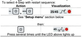
If 4-step restart is enabled from the setup menu the following sequence will occur for steps 3 and 4 (steps 1 and 2 are not altered by the restart option):
