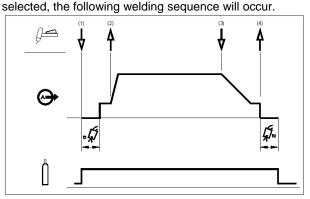
Press and hold the TIG torch trigger to start the sequence. The machine will open the gas valve to start the flow of the shielding gas. After the preflow time, to purge air from the torch hose, the output of the machine is turned ON. At this time the arc is started according to the selected welding mode. After the arc is started the output current will be at the Start current. This condition can be maintained as long as necessary.
