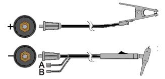
Connect the torch cable to the (-) terminal of the machine and the work clamp to the (+) terminal. Insert the connector with the key lining up with the keyway and rotate approximately ¼ turn clockwise. Do not over tighten.
