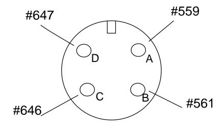
FIGURE B.6 Travel Motor Connector Pins (Older Units with Powered Field.)
