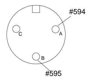
FIGURE B.5 Travel Motor Connector Pins
