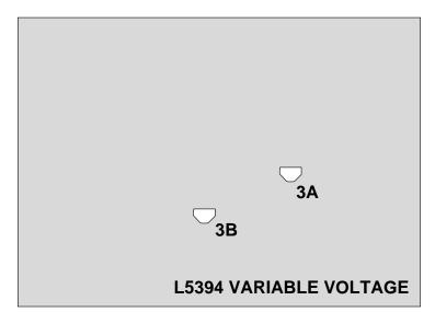
FIGURE B.2 Voltage P.C. Board LED Locations
