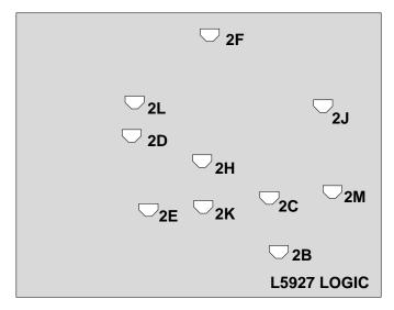
FIGURE B.1 Logic P.C. Board LED Locations
