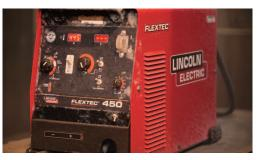
Among other tests, the Flextec<sup>™</sup> 450 was subjected to extreme temperature environmental testing, including heat, cold, humidity, rain and dust.
