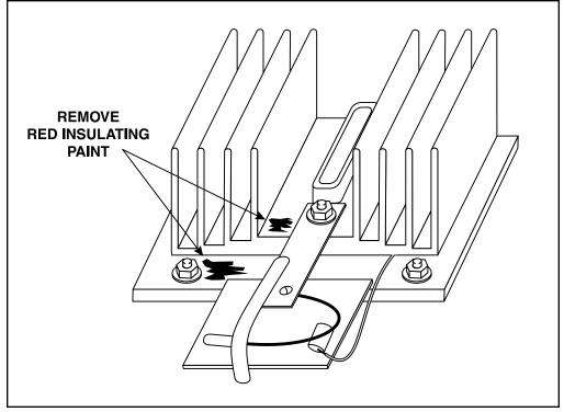
FIGURE F.13 - Heat Sink Test Points.
