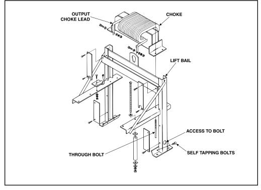
FIGURE F.22 Transformer Bail Assembly Removal
