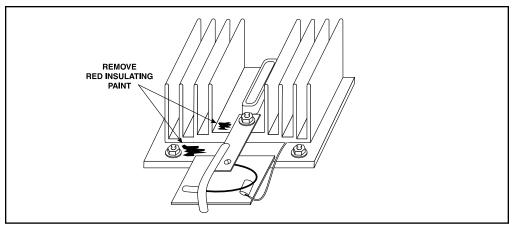
FIGURE F.16 - Heat Sink Test Points.
