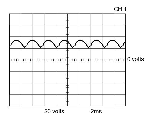
This is the typical DC open circuit voltage waveform generated from a properly operating machine. Note that each vertical division represents 20 volts and that each horizontal division represents 2 milliseconds in time. The machine was loaded with a resistance grid bank. The grid bank meters read 200 amps at 28VDC.
