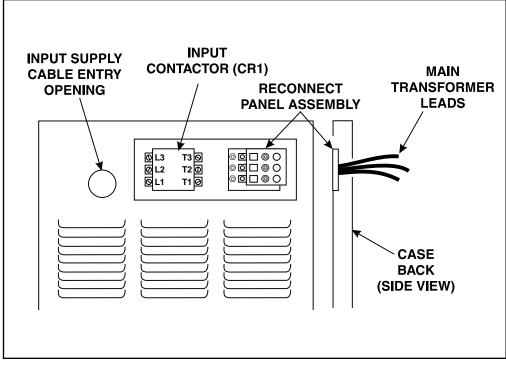
FIGURE F.3 - Input Contactor, Reconnect Panel, and Primary Leads to Main Transformer Locations
