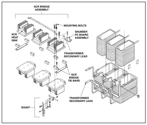
FIGURE F.20 - SCR Output Bridge Removal
