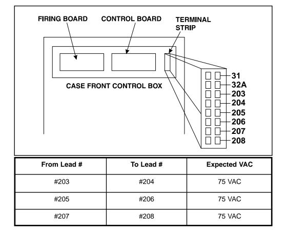
Figure F.5 - Phase Angle Windings Test Points and Terminal Board location.
