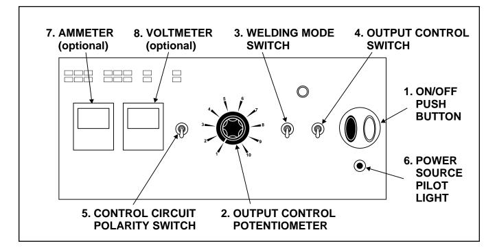
FIGURE B.1 - CONTROL PANEL KEYS
