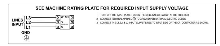
FIGURE A.7-Reconnect Panel Board Positions for Single Voltage Machines
