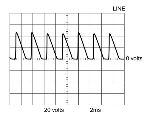
This is the typical DC open circuit voltage waveform generated from a properly operating machine. Note that each vertical division represents 20 volts and that each horizontal division represents 2 milliseconds in time.
