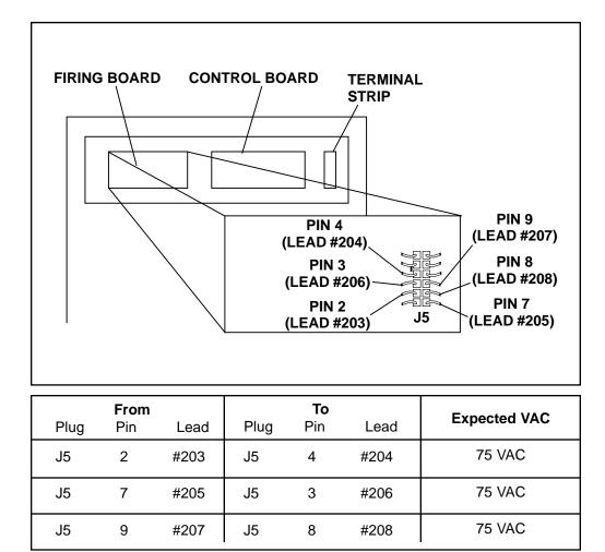
FIGURE F.6 - Phase Angle Windings Test Points and Firing Board Location.
