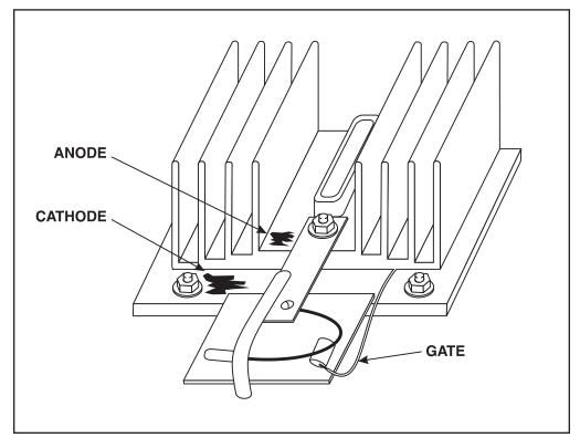
FIGURE F.14 - SCR 1 Test Points.
