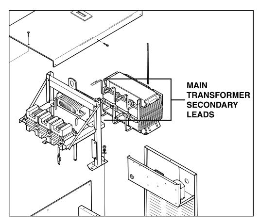
FIGURE F.4 - Main Secondary Lead Test Points.
