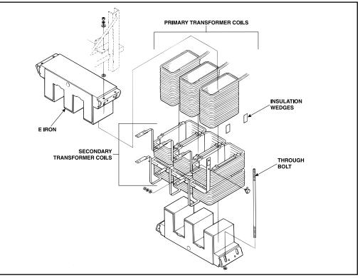
Figure F.23 Transformer coil removal.
