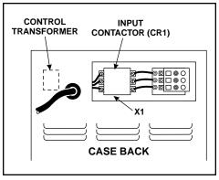
FIGURE F.18 - Input Contactor Cleaning and Removal
