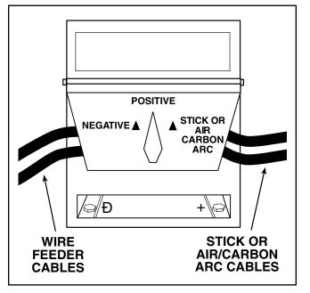
FIGURE C.1 - MULTI-PROCESS SWITCH
