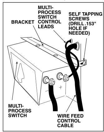
FIGURE C.3 - ATTACHING THE MULTI-PROCESS SWITCH BRACKET.
