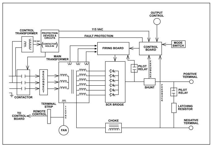
FIGURE E.1 Block Logic Diagram
