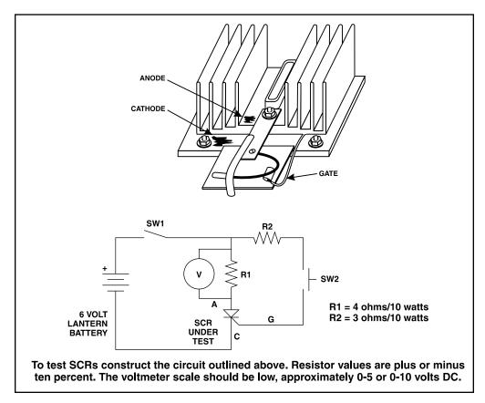
FIGURE F.17 - SCR Tester Circuit and SCR connections.
