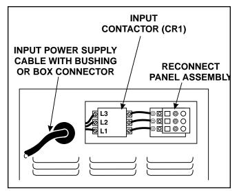
FIGURE A.3 - Input Power Supply Connections
