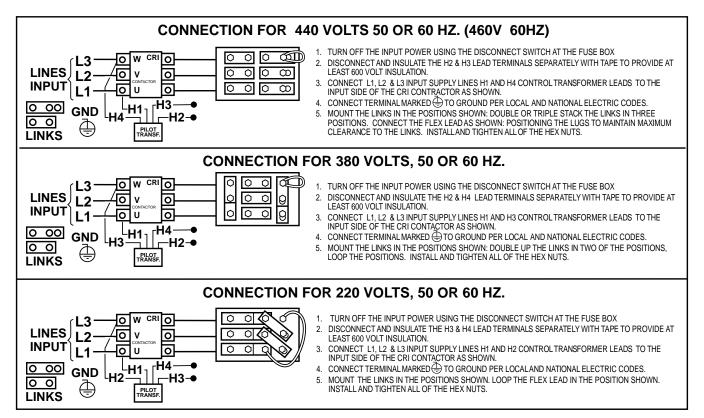
FIGURE A.5-Reconnect Panel Board Positions for 220/380/440 VAC Machines
