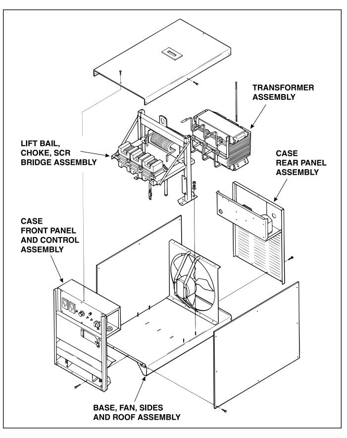
FIGURE D.1 - General Assembly Exploded View
