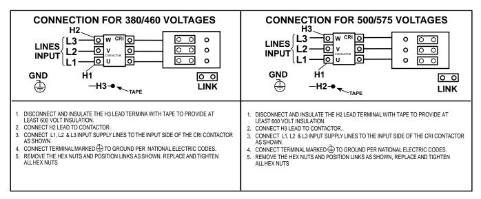
FIGURE A.6-Reconnect Panel Board Positions for 380/460, 500/575 VAC Machines
