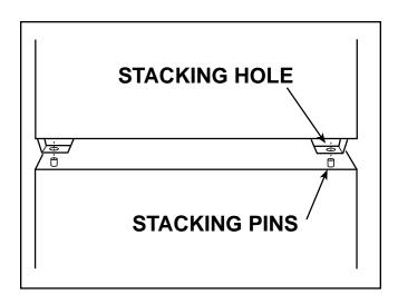
FIGURE A.1 - Stacking IDEALARC DC-600 machines
