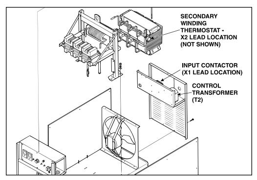
FIGURE F.1 - Control Transformer and Lead Locations
