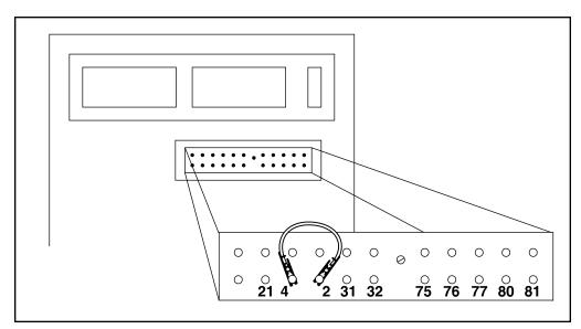
**FIGURE F.8 - Jumper Wire Connection Points**
