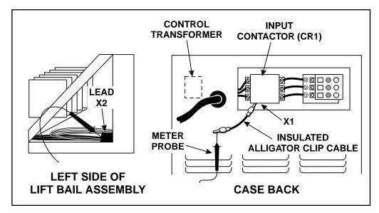
FIGURE F.2 - Control Transformer X1 and X2 Test Connections
