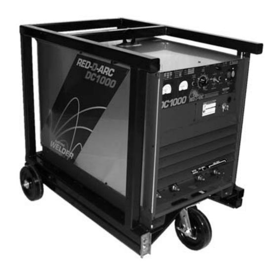
Rugged Tubular Pak-Lok-Frame™ Extreme-Duty™ Stainless Steel Construction 1000 amps DC at 44 volts and 100% Duty Cycle Submerged Arc (SAW), Flux-Cored (FCAW-SS/GS) Gouging (CAC-A), Stick (SMAW) and MIG (GMAW)
